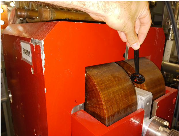
Figure 3: BBBD1. The polarity of the left pole is denoted 'red'. The beam direction in this photograph is from right to left.
